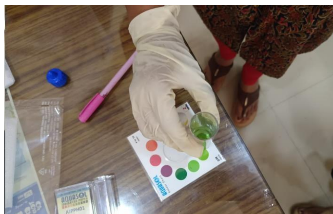
Exhibit 2: pH testing of water – matching the colour with the comparator
